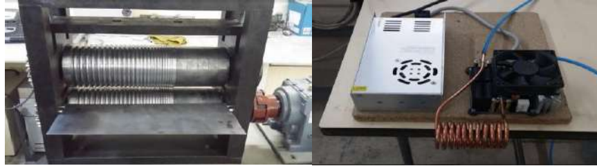
Figure 2. Roll forming machine and induction heating system.
