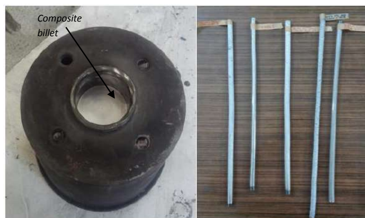
Figure 1. Billets and samples a) Billet in the extrusion cartridge b) Extruded samples
