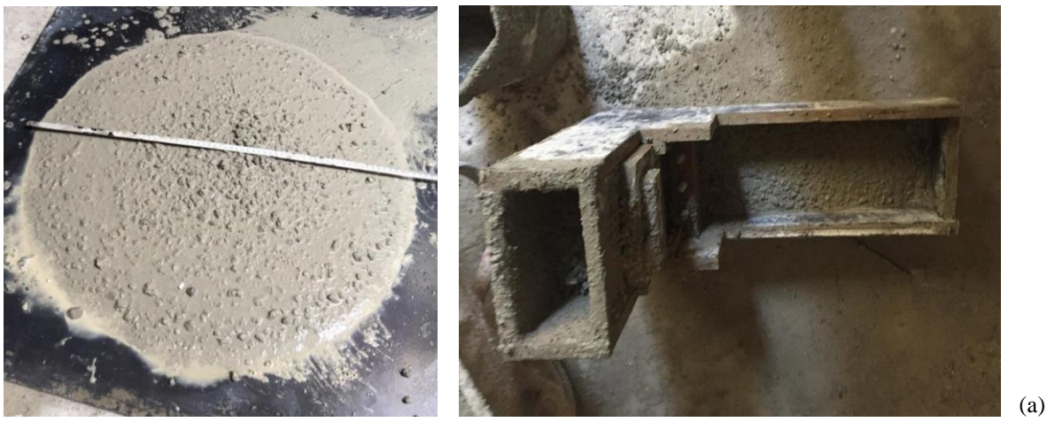
Figure 2.1 a) Slump Flow test b) L box blocking test
